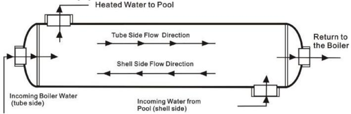
Titanium Pool & Spa Heat Exchangers should be installed downstream of the filtration and pumping equipment. The boiler water must be assisted and the usual precautions taken to prevent air locks. The pool water pump should be controlled by a thermostat in the pool pipe work before the heat exchanger and set at the required temperature.
